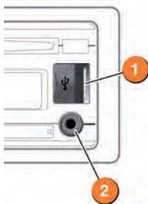
Connect a portable device, then press and release the **SOURCE** button repeatedly until **AUXILIARY** or **USB/iPod** is displayed. MP3 file play will now begin.
