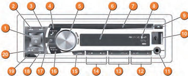
**1. SOURCE:** Press and hold to turn the system on or off. Press repeatedly to switch between **TUNER, DISC, USB AUDIO/iPod, AUXILIARY** and with the telephone option fitted, **BT AUDIO**.
