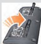
To create a flat loading area, fold the latches into the floor. Raise the latches before the seat is returned to the upright position. The seatback will not unfold until the latches are in the fully forward position and the seat base is latched in the locked position.
