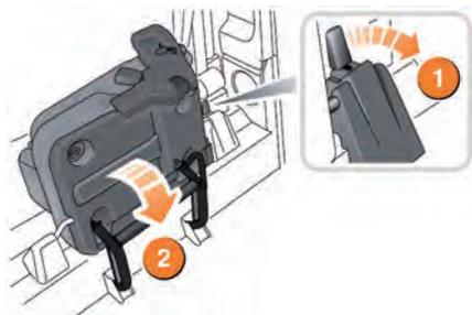
1. Pull the release catch inwards to release the seat assembly.
