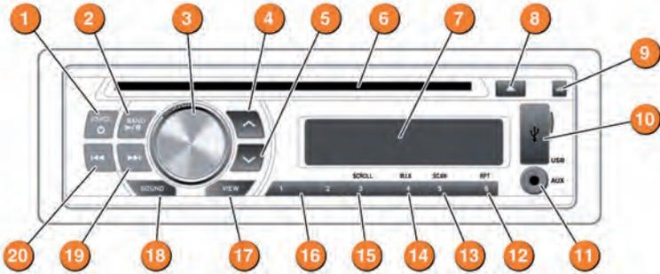
**1. SOURCE:** Press and hold to turn the system on or off. Press repeatedly to switch between **TUNER**, **DISC**, **USB AUDIO** and **AUXILIARY**.
