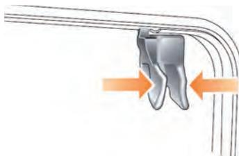
Squeeze the locking mechanism and slide the window to the desired position. Release it and make sure that the window is locked in position.
