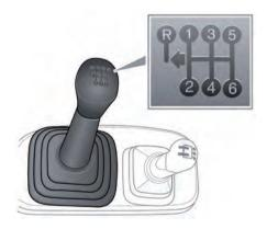
Low range is for very low speed manoeuvring and more extreme off-road conditions where progress cannot be maintained in High range. Some road conditions, such as heavy snow, may also be appropriate for Low range use.
