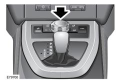
A rotary control just in front of the gear lever is used to select the required special program. When the selector reaches the end of the selection range in either direction it can be rotated further, but it has no effect.
