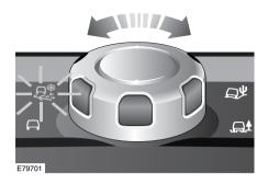
When the starter button is pressed, the indicators around the rotary control are illuminated. The active program is highlighted in amber, and the program icon is displayed in the message centre.
