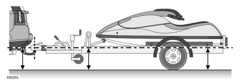
To maintain vehicle stability, it is essential that the trailer is loaded so that it remains parallel to the ground. This is particularly important when towing twin axled trailers.
