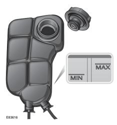
Ensure the coolant level is maintained between the level indicator marks located on the side of the expansion tank.
