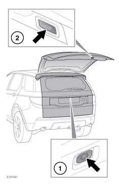
1. Press the button to open the powered tailgate. The button can also be used to stop, reverse the direction, or close the tailgate.
