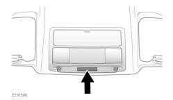
The warning lamp, mounted in the roof console, will display the operational status of the passenger front airbag, as shown in the following table.
