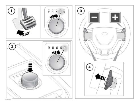
The rotary gear selector rotates in either direction. At engine start-up, the gear selector elevates out of its parked position.
