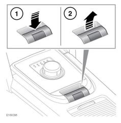
1. With the ignition turned on, press the brake pedal, then press down and release the EPB switch. This will release the EPB.
