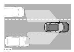
The Blind Spot Monitor (BSM) system monitors a zone that covers the area adjacent to the vehicle, that is not easily visible by the driver and is designed to identify any object overtaking the vehicle. The system uses a radar on each side of the vehicle to identify any overtaking vehicle/object within the blind spot area of the vehicle, while disregarding other objects which may be stationary or travelling in the opposite direction, etc.
