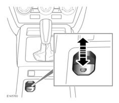
With the ignition turned on, press the brake pedal and press down on the EPB switch. This will release the EPB.
