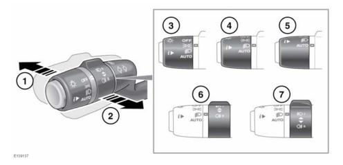
With the headlamps on, push the control away from the steering wheel to select high beam. The warning lamp will illuminate. See 36, HIGH BEAM (BLUE).
