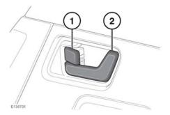
From inside the vehicle, all of the doors can be locked by pressing either the driver or passenger lock lever (1).
