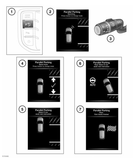
To activate, press the Park assist button while driving forwards at less than 18 km/h (11 mph). The Park assist button indicator will illuminate.
