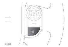
Press the button to turn the heating steering wheel feature on and off. An amber indicator will illuminate when the heated steering wheel feature is on.
