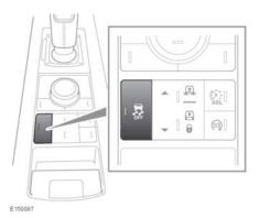
To disable DSC, press and briefly hold the DSC OFF switch. The DSC OFF warning lamp will illuminate (see **50**, **DYNAMIC STABILITY CONTROL (DSC) OFF (AMBER)**). Deactivating DSC also reduces the level of Traction control intervention and may lead to an increase in wheel spin.
