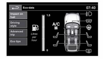
The Eco-data system is designed to help the driver maximise fuel economy by providing vehicle data and driving tips. The Eco-data system can be accessed through the **Extra features** menu in the Touch screen. See **74**, **EXTRA FEATURES**
