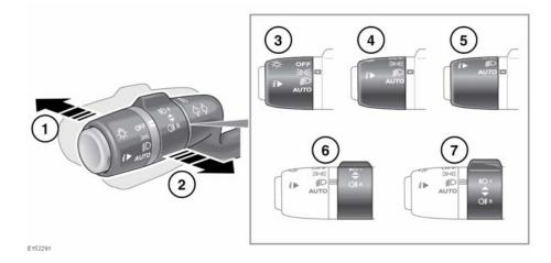
With the headlamps on, push the control away from the steering wheel to select high beam. The warning lamp will illuminate. See 51, HIGH BEAM (BLUE).
