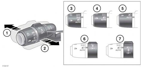
With the headlamps on, push the control away from the steering wheel to select high beam. The warning lamp will illuminate. See 70, HIGH BEAM (BLUE).
