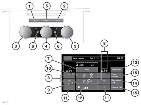
There are 2 types of rear climate control: 3 Zone and 4 Zone. All of the 3 zone controls will affect the whole of the rear passenger compartment. The 4 Zone allows independent control of each side.
