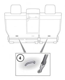
For child seats fitted with **non-rigid** LATCH connectors, connect the lower tether strap hooks to the anchor bars and tighten the straps.
