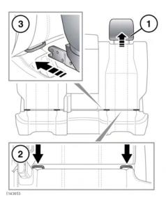
LATCH anchorage child restraints can only be fitted to the outer seat positions on the second row of seats.
