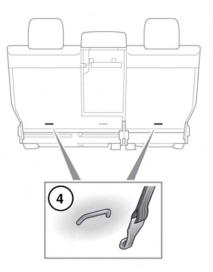
For child seats fitted with **non-rigid** LATCH connectors, connect the lower tether strap hooks to the anchor bars and tighten the straps.
