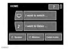
Use the left/right screen select keys on the rear media remote control, or the front touch screen controls, to allow further options to be set and selected.
