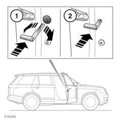
In the event of the battery discharging or a fault with the keyless locking system, the doors must be locked manually.
