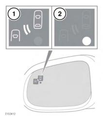
The Blind Spot Monitor (BSM) system monitors a zone that covers the area adjacent to the vehicle, that is not easily visible by the driver and is designed to identify any object overtaking the vehicle (3).
