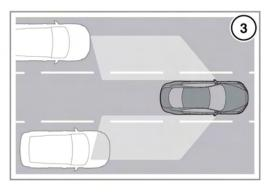
The system uses a radar on each side of the vehicle to identify any overtaking vehicle/object within the blind spot area of the vehicle, while disregarding other objects which may be stationary or travelling in the opposite direction, etc.
