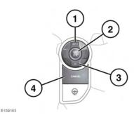
SET+: Press to set the speed or to increase the set speed. The cruise control warning lamp will illuminate to confirm cruise control is operational (see 70, CRUISE CONTROL (GREEN)).
