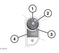
SET+: Press to set the speed or to increase the set speed. The cruise control warning lamp will illuminate to confirm cruise control is operational (see 70, CRUISE CONTROL (GREEN)).
