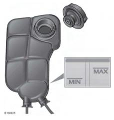
Ensure the coolant level remains between the level indicator marks located on the side of the expansion tank.
