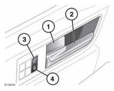
From inside the vehicle, all the doors can be locked by pressing either the driver or passenger lock lever (1).
