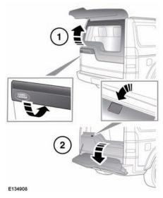
**Upper tailgate:** Unlock the vehicle and press the touchpad (1) on the underside of the exterior handle. Pull the tailgate upwards to open.
