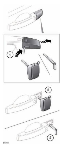
Insert the key blade into the slot at the base of the door lock cover and gently lever the key blade upwards.
