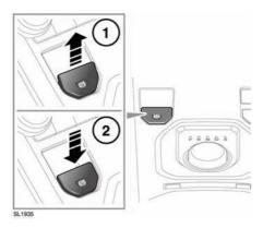
To apply the parking brake, with the vehicle stationary, pull up the lever and release it.
