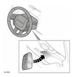
Position the Smart Key against the underside of the steering column cover with the buttons facing downwards.
