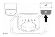
To disable DSC, press and briefly hold the DSC OFF switch. The DSC OFF warning lamp will illuminate continuously. The amber DSC OFF warning lamp in the instrument panel will also illuminate. Deactivating DSC also reduces the level of Electronic Traction Control intervention and may lead to an increase in wheel spin.
