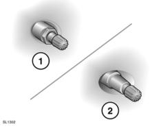
Wheels fitted with TPMS can be visually identified by the external metal lock nut and valve (1). All Land Rover non-TPMS wheels have a rubber valve fitted (2).
