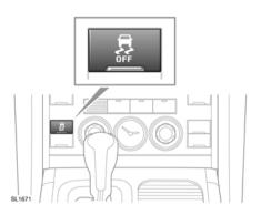
To disable DSC, press and briefly hold the DSC OFF switch (the DSC OFF warning lamp will illuminate continuously). Deactivating DSC also reduces the level of traction control intervention and may lead to an increase in wheel spin.
