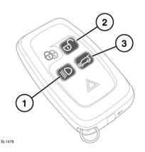
To raise the vehicle, press and hold buttons **1** and **2** simultaneously
