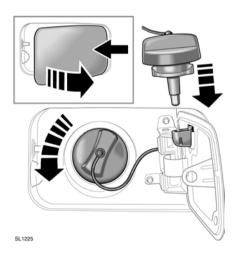
The gas cap flap is located on the right-hand side of the vehicle, at the rear.
