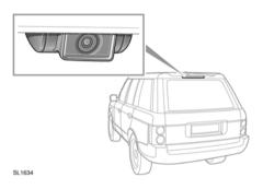
When Reverse gear is selected, the touch screen automatically displays the view to the rear of the vehicle.
