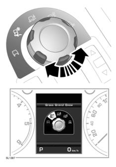
A rotary control just in front of the gear lever is used to select the required special program.
