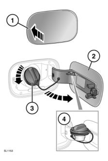
The fuel filler flap is located on the right-hand side of the vehicle, at the rear.
