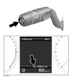
A short press (1 second or less) or a series of short presses of the i button will change the trip computer display.
