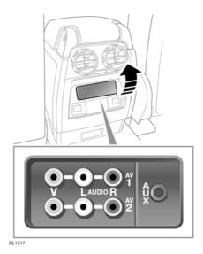
The 3.5mm AUX socket allows additional equipment (e.g. personal stereo, MP3 player, hand-held navigation unit, etc.) to be connected to the audio system.
