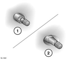
Wheels fitted with TPMS can be visually identified by the external metal lock nut and valve (1). All Land Rover non-TPMS wheels have a rubber valve fitted (2).
