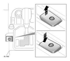
With the vehicle stationary, pull up the lever (arrowed) and release it.
