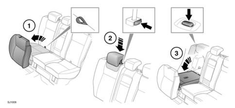
The split folding rear seat can be folded completely to accommodate large loads, or partially to accommodate large loads and still retain seating for passengers.
