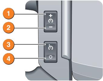
Cruise control will automatically **disengage** when the **brake pedal** is used or when the vehicle speed falls below 30 km/h (18 mph).
