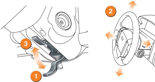
1. Move the lever located under the steering wheel fully downward.
