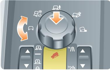
The Terrain Response system is always active and cannot be switched off. When the vehicle is started the system will normally start in the **General** program.
