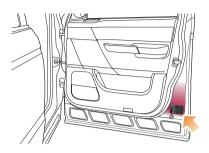
The correct tyre pressures are shown on a label attached to the driver's door.
