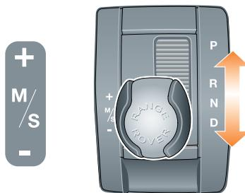
1. Select Sport mode. The transmission will automatically select the gear most appropriate to the vehicle's road speed and accelerator position.
