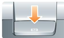
The starter switch must be in position **I** or **II**. Apply the foot brake and press down on the parking brake lever. If the vehicle is stationary with the parking brake applied and either **D** (Drive) or **R** (Reverse) selected, pressing the accelerator will automatically release the parking brake.
