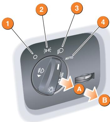
Fog lamps cannot be operated if the lamps master switch is in **AUTO**.
