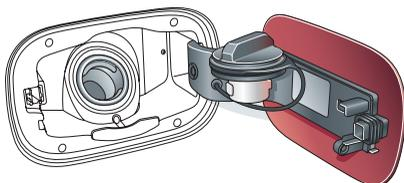
The filler cap is secured to the vehicle by a strap. For your convenience, a holder is provided on the flap to store the cap whilst refuelling.
