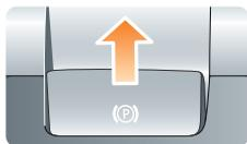
With the vehicle stationary, pull up the parking brake lever and then release it. The lever will return to a neutral position and the red warning indicator in the instrument pack will illuminate.
