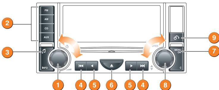
1. Press to switch audio unit on/off and rotate to adjust the volume.
