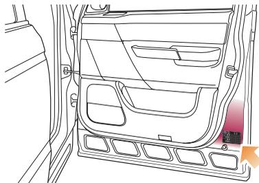
The correct tyre pressures are shown on a label attached to the driver's door.
