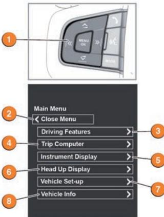
A number of vehicle features and display settings may be configured via the Instrument panel menu.
