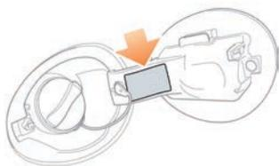
The fuel filler flap is located on the right side of the vehicle. If the vehicle is locked, the filler flap cannot be opened.
