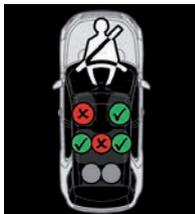
An audible warning will sound if a seat belt is unfastened while the vehicle is moving.
