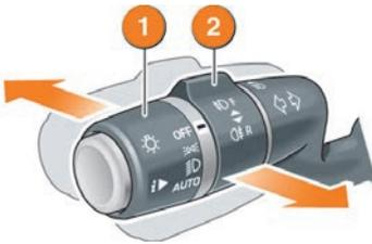
1. **Outer collar.** Rotate to first position for side lamps, second position for headlamps, and the third position for **AUTO**. With **AUTO** selected, all exterior lamps switch on automatically when the ambient light fades.
